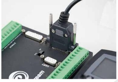
Figure 3-3 Switch to NV MPG mode
