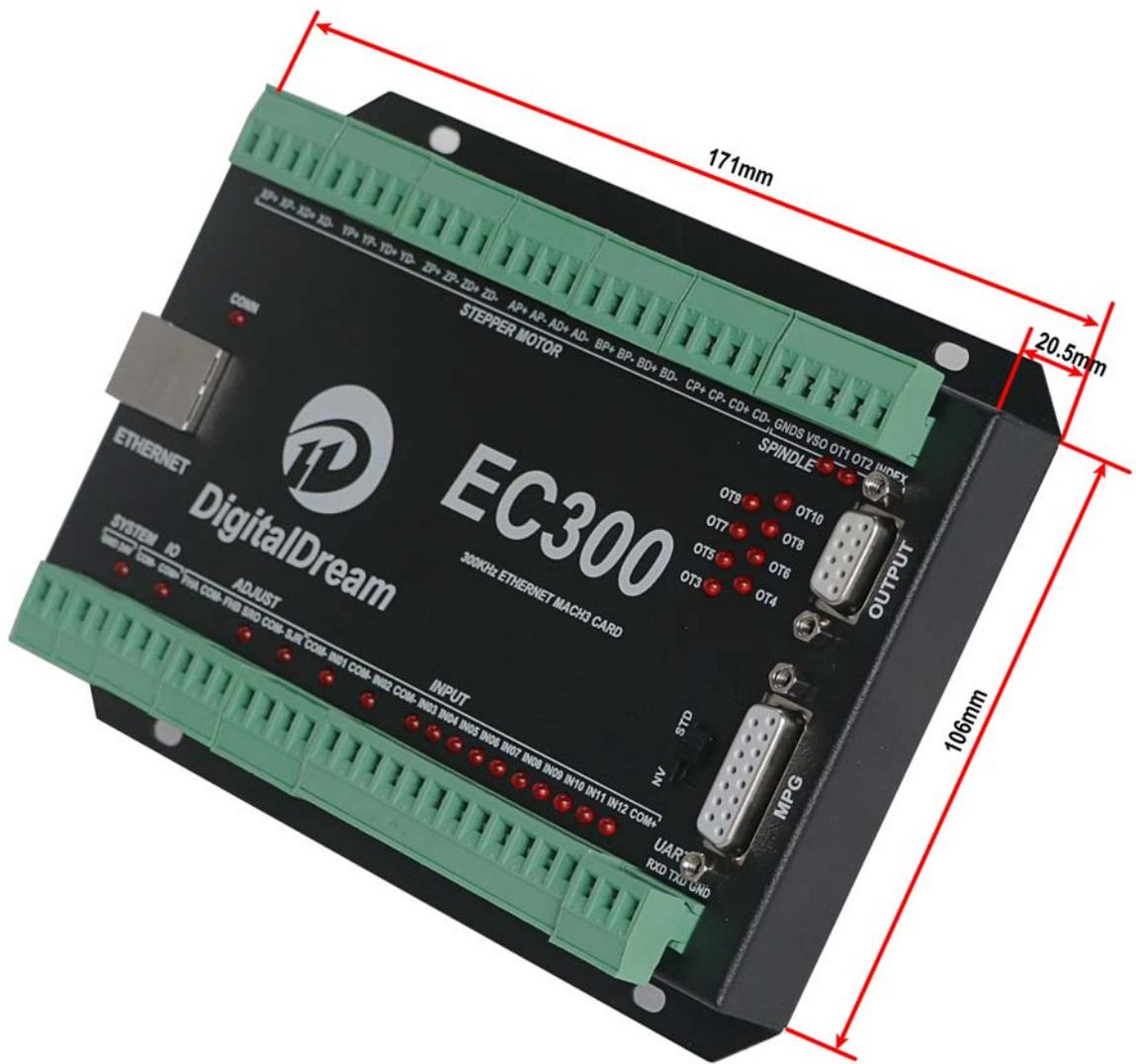
Figure1-1. EC300V5 front appearance and size
