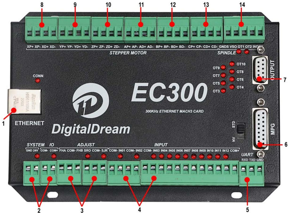
Figure2-1. Product wiring section and interface summary
