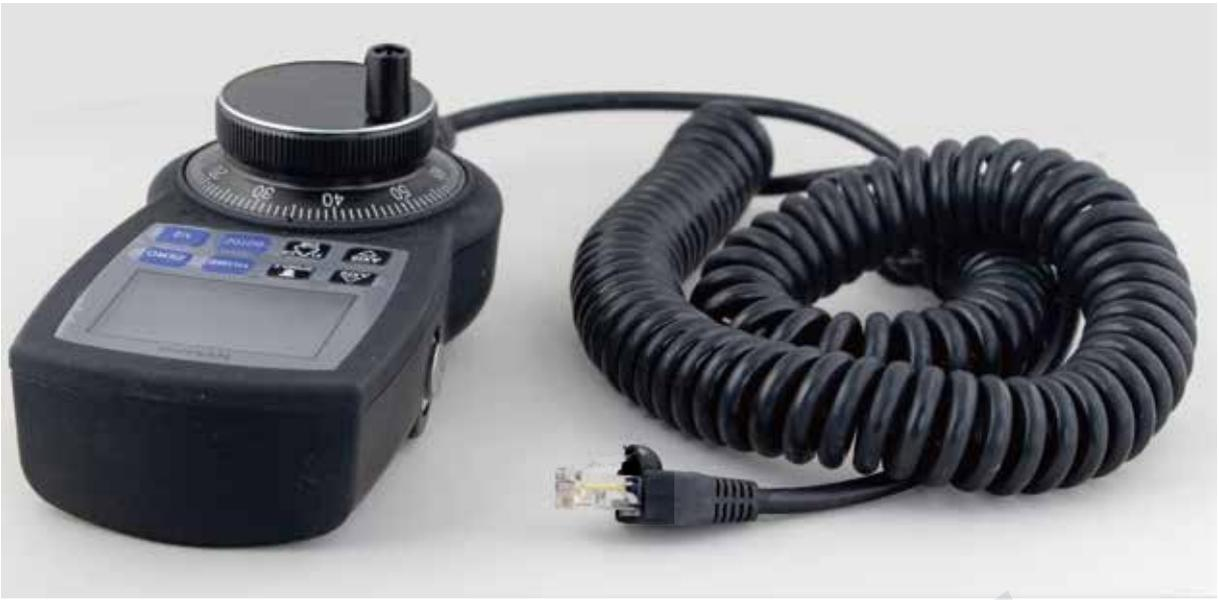
Figure 1-4 RJ45 wiring cable
