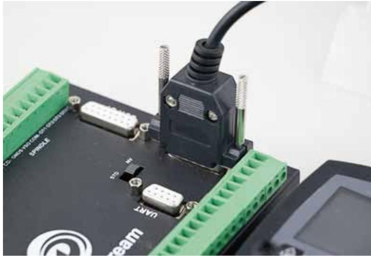
Figure 3-3 Switch to NV MPG mode
