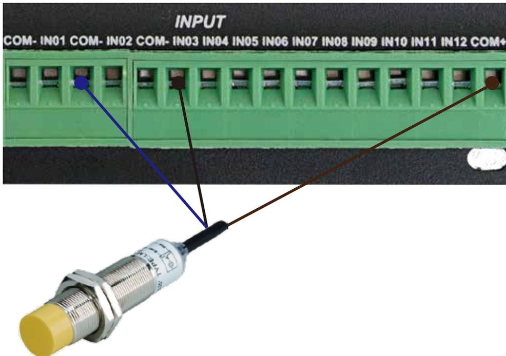
Figure 5-12 NPN 3 lines Proximity Switch Connection Example
