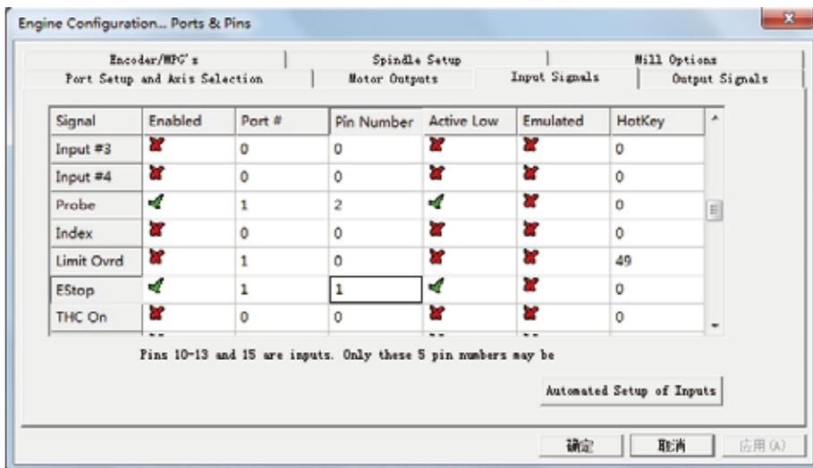
Click “Spindle Setup” switch to the spindle settings page.
