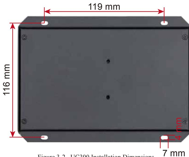
Figure 3-2 UC300 Installation Dimensions
