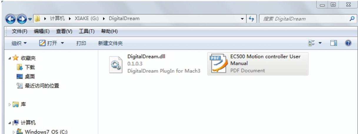
In your computer which you will run the UC300 controller, you must already installed the Mach 3 Software, and now pls copy the PlugIn in to C:\Mach3\PlugIn. (If the user install the Mach 3 software in C-disk.)
