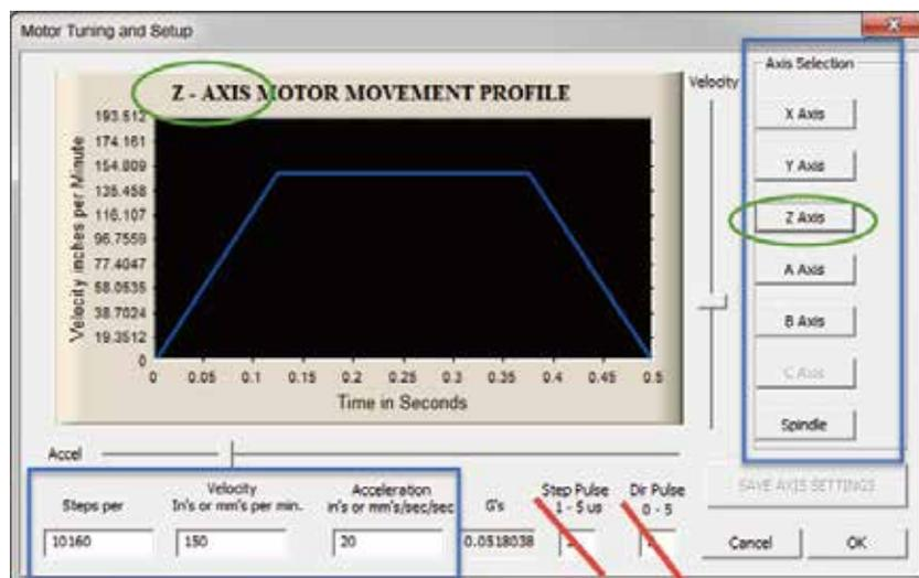
Mach3's Menu -> Config -> Motor Tuning (and Setup).
