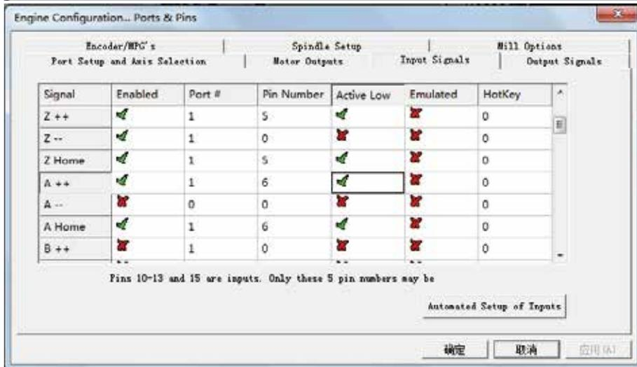
Here you can configure according to your actual needs the corresponding function. Optional Function include XYZABC 6axis's Upper and lower limit、XYZABC 6axis's HOME point. We set upper limit and home of XYZA to 3456 corresponding IN3/IN4/IN5/IN6 of the Controller board.
