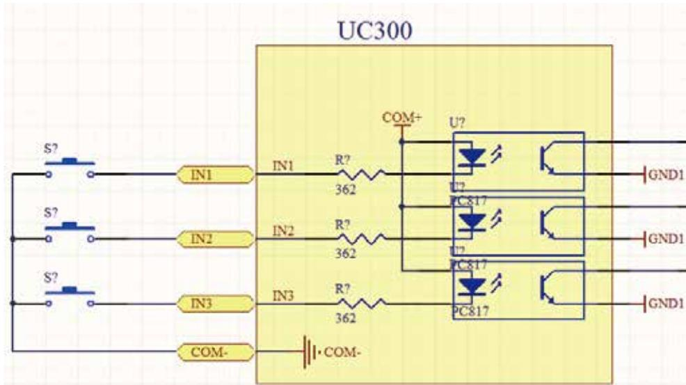
Figure 5-10 Probe/Estop/ and other switch input connection
