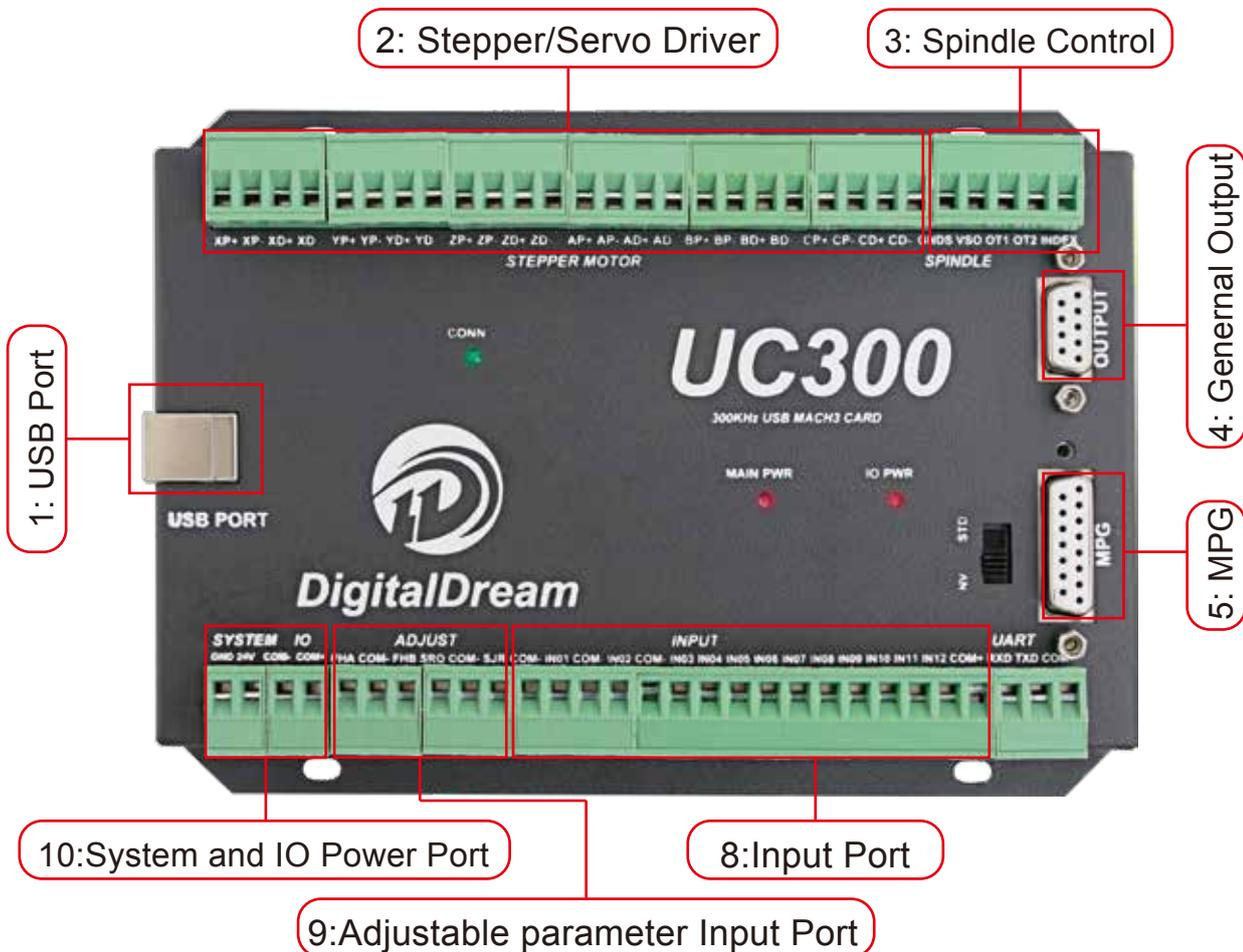
Figure 5-1 UC300 Wiring Over-view
