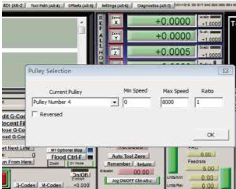
Figure 5-4 UC300 Spindle Motor Max Speed Setting
