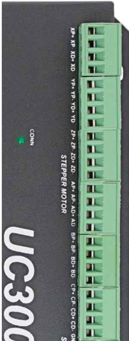
As the Marked No. 2 from Figure 5-2,there is the Stepper/Servo Interface.The device can be used to control machine tools with stepper or servo motor controls with pulse and direction signals.The option for users is 3-6 axis.
