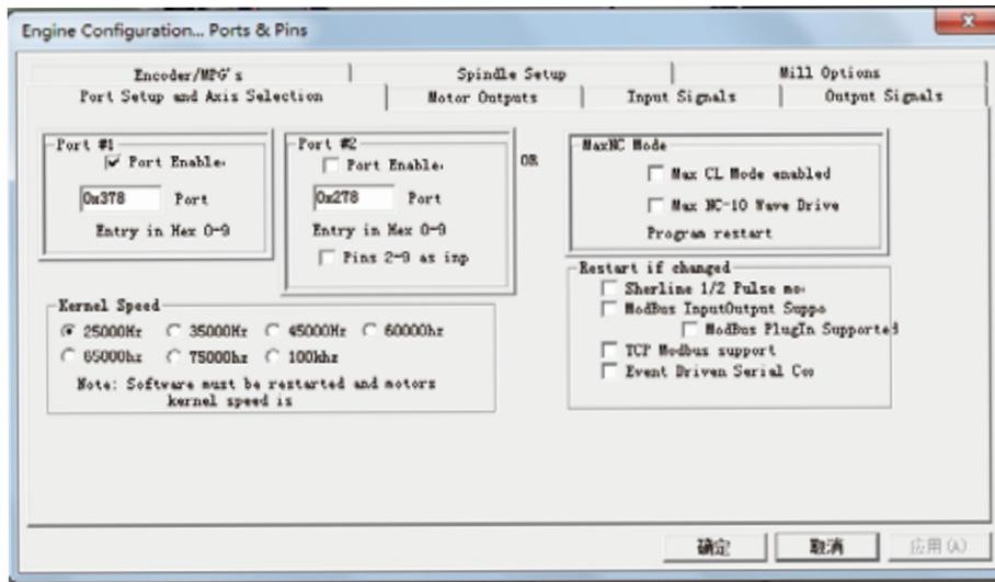
Then go to Right Lables: Motor Outputs and start to configurate as below:
