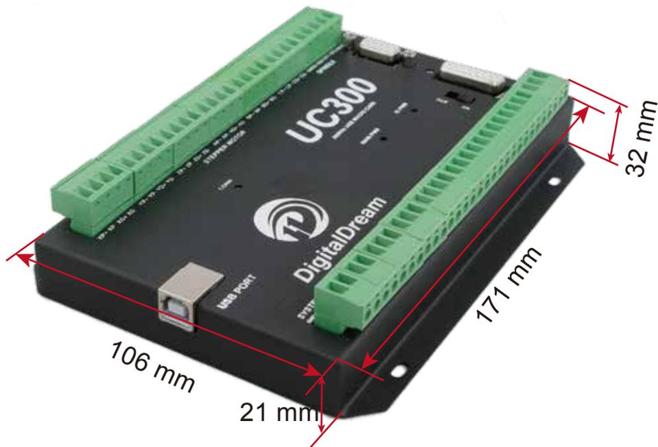
Figure 3-1 UC300 Front Appearance and size
