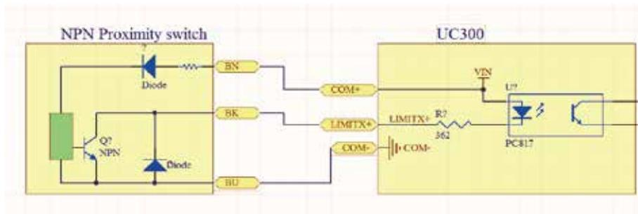
Figure 5-11 Probe/Estop/ and other switch input connection
