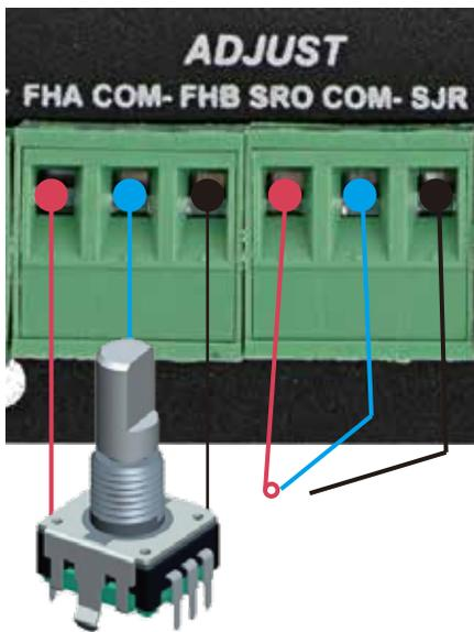
From the Figure 5-1 shows, the Marked No. 9 is for adjustable input interface, which must be operated by the digital potentiometer. The interface will make us to operate the FRO, SRO and SJR very Easy and convenient. The Interface should be operated with position switch and digital potentiometer, for the FRO, SRO and SJR adjustment.
