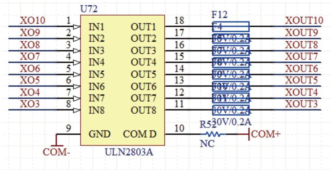
Figure 5-6 OUTPUT port internal structure
