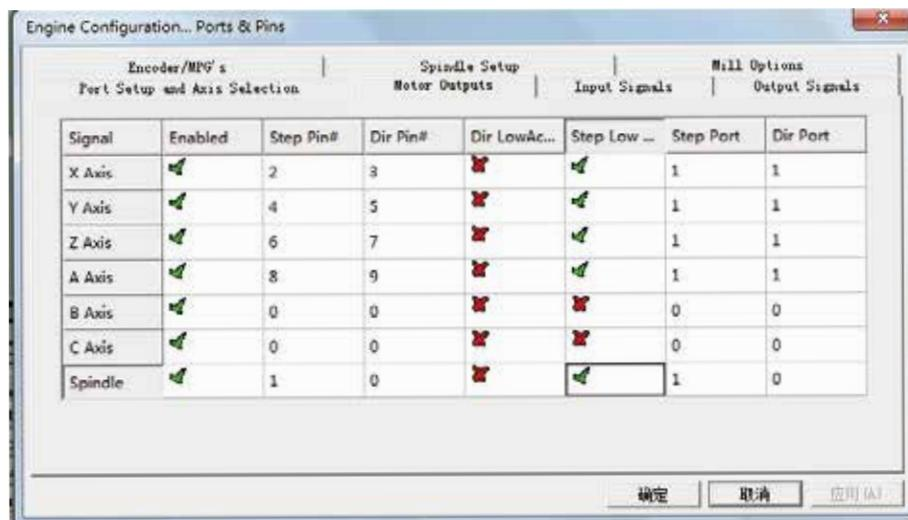
This page is to select the stepper motor control pins. Because Stepper motor control pins address are fixed by the controller board, So here only need to define the Pin address(No.s),we can define other parameters meter. To make sure the Z axis to the right direction(Up is '+',down is '-'), Z axis's "Dir low" should be set to "✓". Other axes's should be set as the user's request.
